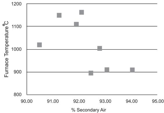
Figure 5: Effect of %Secondary Air on Furnace Temperature (Mesh Size 150).
