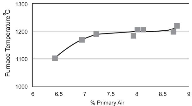
**Figure 4: Effect of % Primary Air on Furnace Temperature (Mesh Size 200).**
