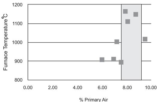
**Figure 3: Effect of Primary Air on Furnace Temperature (Mesh Size 150).**
