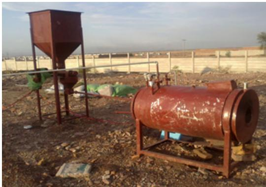
**Figure 1: The cyclone combustor test rig.**
