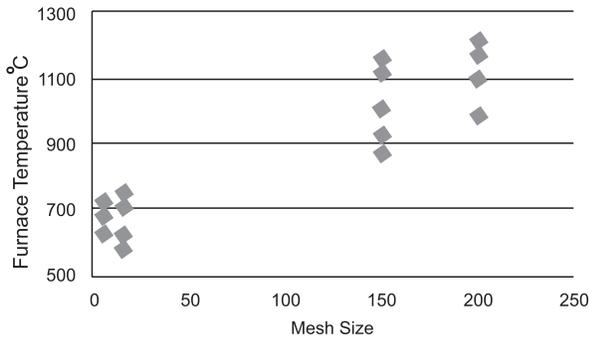
**Figure 2: Effect of Mesh Size on Furnace Temperature.**
